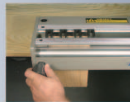
above The wood is clamped vertically in the jig
