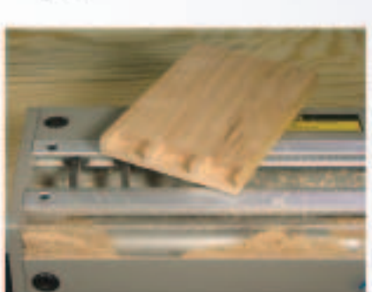
above The finished dovetail pins
