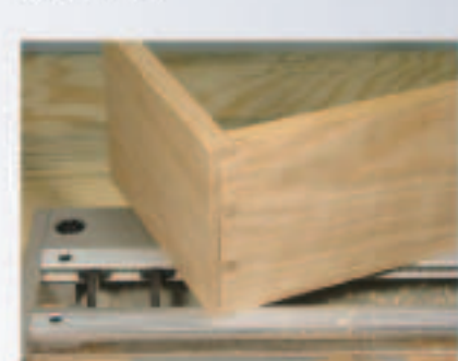
above The completed half blind dovetail jig
