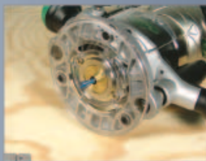
above With guide-bush and dovetail bit fitted. The depth of cut is set
